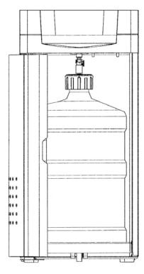
**NOTE:** If there is not a secure connection between the hose cap and the connector on the water cooler, the water pump will operate but the water cooler will not dispense water. Make sure the hose is connected to the water cooler correctly.
